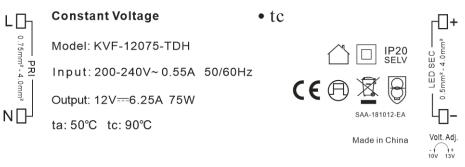
%Input (L) and (N) with wire to be connected with AC
