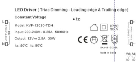
%Input (L) and (N) with wire to be connected with AC
